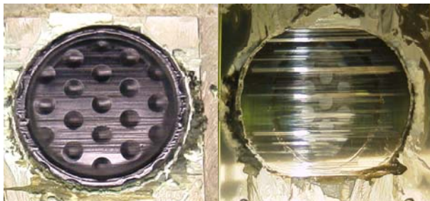
pict. 3: shape of MSM® after a sliding path of 50,000 m
